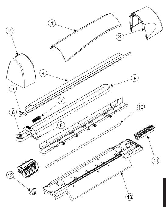
Figure 6-1. Croma24 Assembly Parts (Platen and Above).
